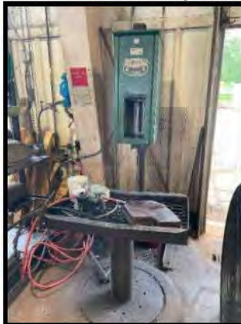
Picture 32: Indoor Used Oil Separator and Oil Filter Crusher – 8/13/2024
